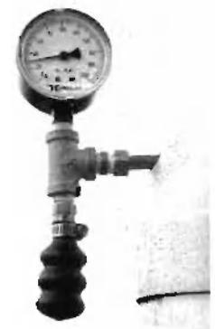
Air pressure gauge to show tank water level.
