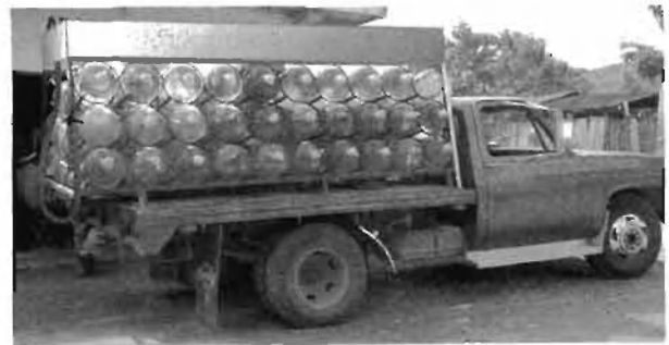
Stainless steel water tank/bottle truck proposed for distribution of inexpensive, bulk drinking water refills for an Indian village in Mexico. 27
