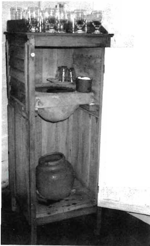
Old-fashioned drinking water filter/cooler in a farmhouse in rural Cuba. The owners pour raw water into the depression in the porous carved stone filter. From there, it drips into the clay storage urn. Louvered vents provide evaporative cooling.
