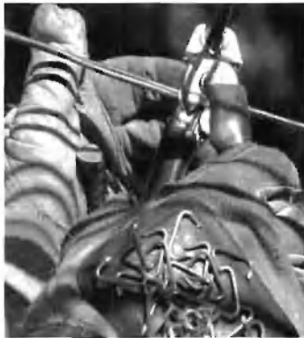
Hog ring pliers and cool magnetic glove loaded with rings.
